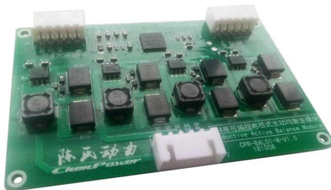
3/4串可编程电感式主动均衡主模块 3/4 series programmable inductive active balance module CPR-BAL01-M/4S
